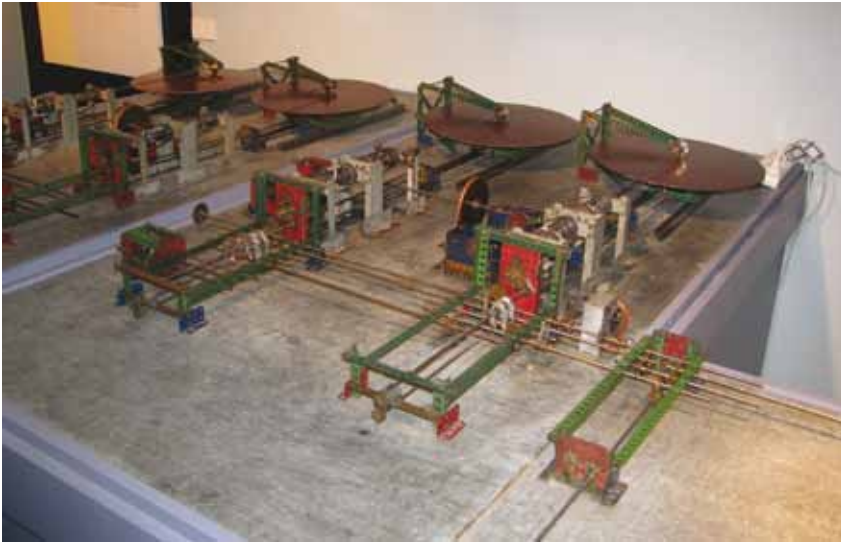
The Differential Analyser (analogue computer) used by Lennard-Jones is now in the Museum of Transport and Technology, Auckland, New Zealand. (The Walsh Memorial Library, Museum of Transport and Technology, New Zealand.)
